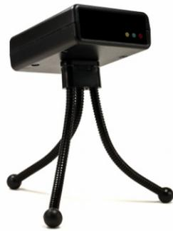
**2** Connect the Vmarker IR-sensor USB with the supplied USB cable to a free USB port of your computer and wait until the red LED on the sensor is continuously lit.
