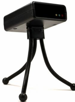
Point the Vmarker sensor II with the front (the side of the LEDs) to the projection surface.
